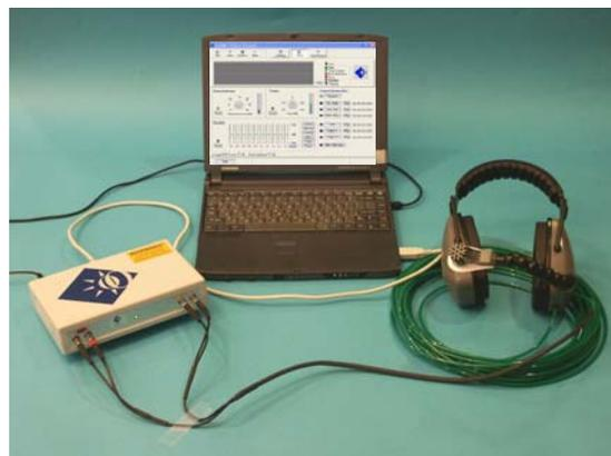
System includes: dual-channel microphone and fiber optics (in MR room), electro-optic unit and software (in the control room)
